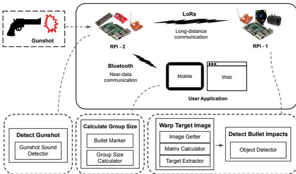
Fig. 1. Block Diagram of Proposed Module
